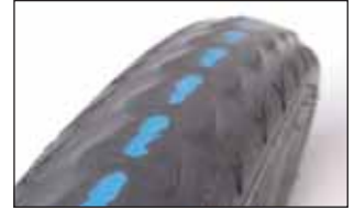
The puncture protection layer can be seen. The tire must be changed urgently.
