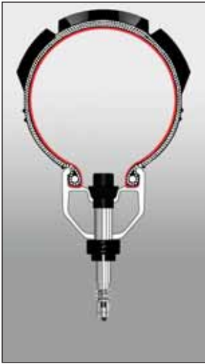
Tubeless System: Airtight seal between tire and rim.
